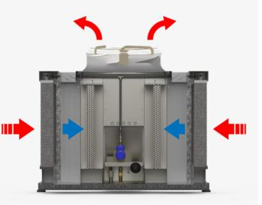
When the outside temperature rises, the PLC activates the adiabatic mode. This involves a water tank that fills to an appropriate level, the water pump starts in a closed circuit and feeds the adiabatic panels, the gates that previously allowed bypass passage close, and the fan speeds are reduced to the appropriate level to allow maximum exchange efficiency.
